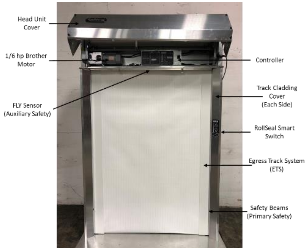
Figure 1: Door Components
