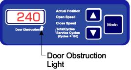
The action of the door when the safety beams are tripped can be controlled by the P20 setting described in Section 6.1
