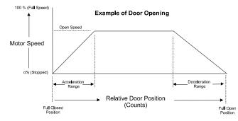
stopped position to the open or close speed. The Deceleration Range is measured in units of counts and is the range over which the door will decelerate from the open or close speed to a stopped position. Typical values for the Acceleration Range are 40 counts and for the Deceleration Range is 80 counts.
