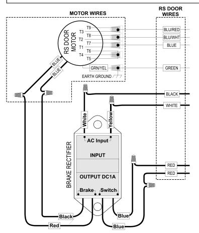
The SC-325/SC-650 Controllers and RS 500/600 Doors can be field upgraded to accommodate either 115 VAC or 230 VAC power supply. If the desired power supply voltage is different from the factory preset/prewired voltage, the appropriate version Brake Rectifier must be ordered separately, field-installed on the RS Door, and the SC Controller switch & jumper settings changed accordingly.
