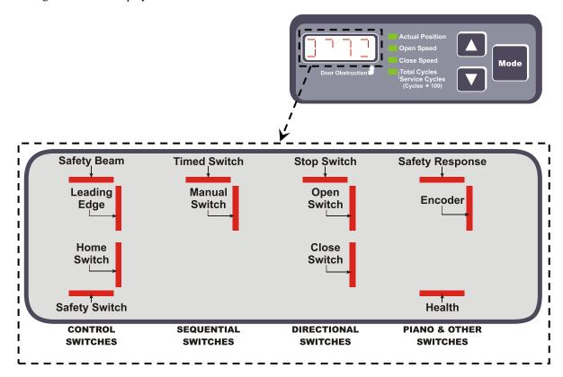
If a display segment is "ON", the switch is Made; Segment is "OFF", switch is Not Made.
