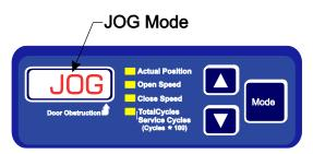
In the Jog Mode the door can be opened and closed and is not
