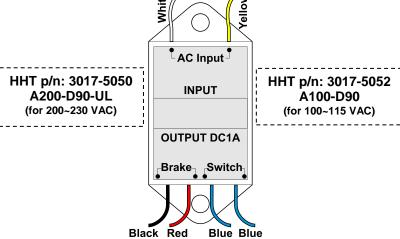
The <u>SC-325 Controllers</u> are factory preset to 115 VAC and the <u>RS-500 Doors</u> factory prewired to require a 115 VAC power supply.
