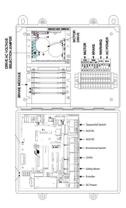
11.2 Smart Controller SC-325 Connection Diagram (Internal Wiring)
