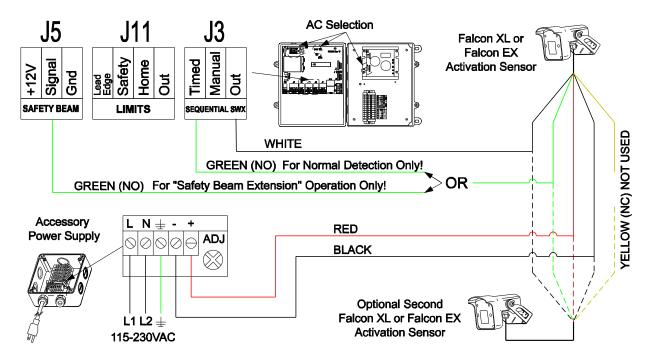
14.4.2 Wiring Falcon IS40 Infrared and Microwave Sensors
