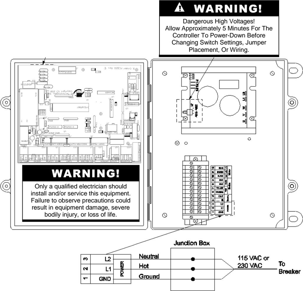
12.2RS-500/600 Motor Brake Rectifier Wiring Diagram
