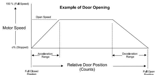
stopped position to the open or close speed. The Deceleration Range is measured in units of counts and is the range over which the door will decelerate from the open or close speed to a stopped position. Typical values for the Acceleration Range are 40 counts and for the Deceleration Range is 80 counts.
