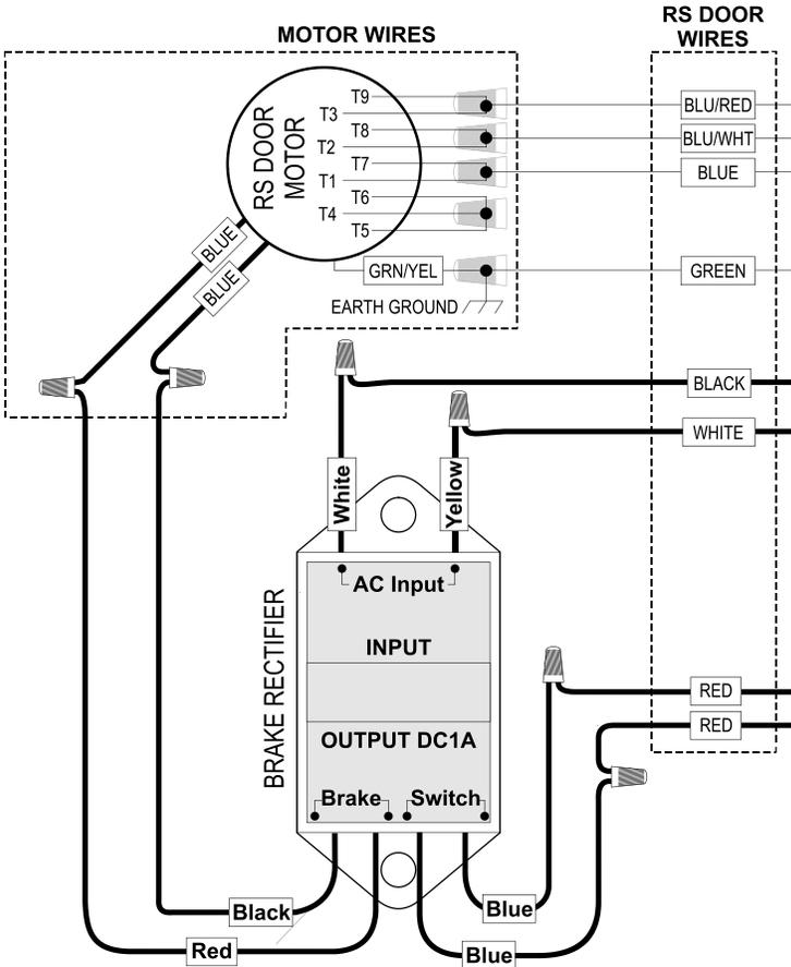
The **SC-325/SC-650 Controllers** and **RS 500/600 Doors** can be field upgraded to accommodate either 115 VAC or 230 VAC power supply. If the desired power supply voltage is different from the factory preset/prewired voltage, the appropriate version Brake Rectifier must be ordered separately, field-installed on the RS Door, and the SC Controller switch & jumper settings changed accordingly.
