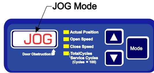
In the Jog Mode the door can be opened and closed and is not affected by the Home limit switch or the Safety beam. Therefore, the operator must carefully watch the door movement when nearing the full open and full closed positions. To exit the Jog Mode, press and hold the **Up** ( $\triangle$ ) and **Down** ( $\nabla$ ) arrow buttons for at least 5 seconds. The controller will return to the normal operating mode with the Actual Position shown in the display.
