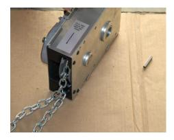
Take the chain hoist up to the shaft protruding from the right side of the door head unit. Rotate the chain so that the keyway in the upper hole matches the keyway position on the shaft. Insert the key from the hardware bag into the keyway of the chain hoist and slide the assembly onto the shaft until it hits the hoist mount on the track.
