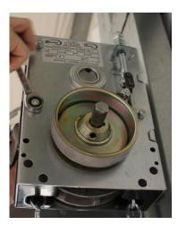
You can now remove the 3/8" bolt and keeper bracket from the drive shaft of the door. The keeper bracket has two 1/4" bolts that will have to be removed from the side of the head.
