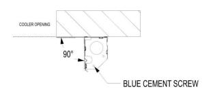
Use a square to ensure that each track is square to the cooler wall face at the bottom. Install a blue cement screw supplied in the hardware kit in the prepunched hole of the bottom brace on each side.
