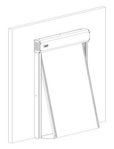
If the emergency egress has been used, the egress tracks will have to be reset to allow the door to seal. In order to reset the front egress tracks, ensure that the panel and the two tension pipes are pushed back into the track cavity. While holding the panel in position, flip each track back into the operational position so that the magnet can seal to the panel. Once the panel and tracks have been reset, the door is ready for operation.
