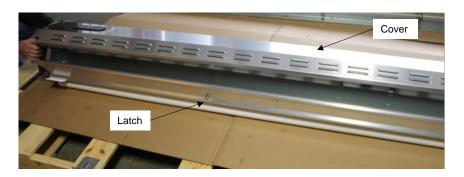
their slots in the frame so that the cover can be removed and set aside with the other cladding until the door frame is installed.
