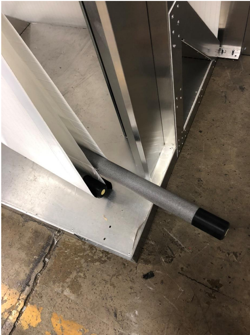
Figure 22: Removal of Tension Pipes
