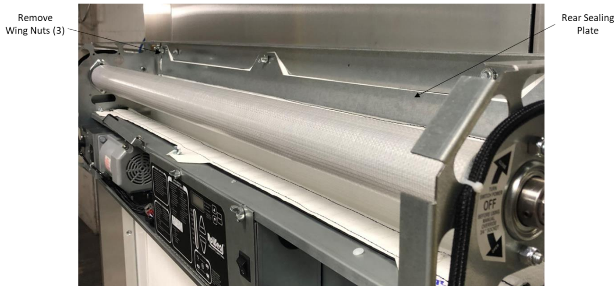
Figure 23: Removal of Rear Sealing Plate
