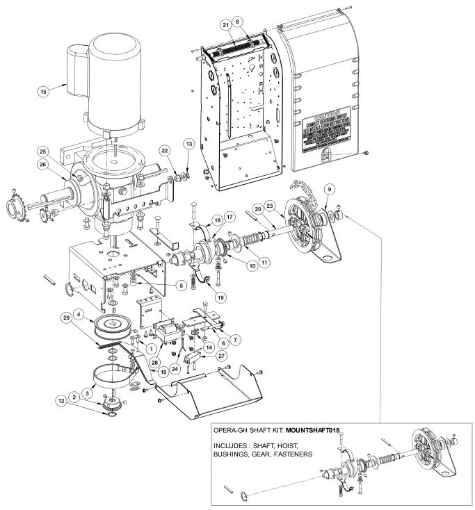
Figure 45 - Opera-GH Mechanical Exploded View
