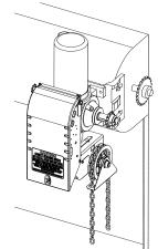
Figure 6 - Right Side Hood Mount with BRACKET111 (Chain Hoist on Right)
