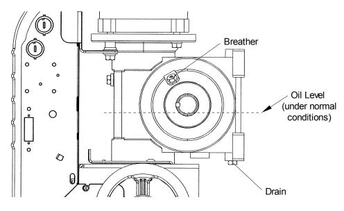
Figure 41 - Gear Reducer Breather
