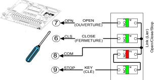
Figure 19 - STATION 079 3-PBS Open / Close / Stop with Key Lock-out
