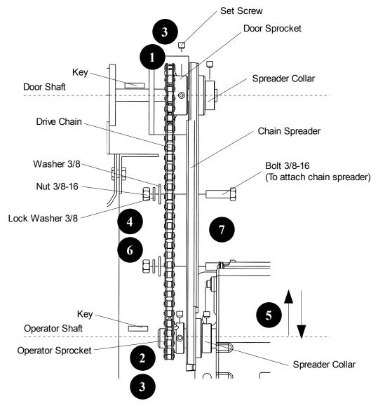
Figure 8 - Hardware Components
