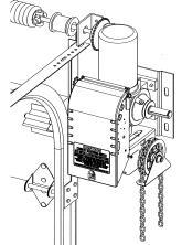
Figure 5 - Right Side Wall Mount with BRACKET112 (Chain Hoist on Right)
