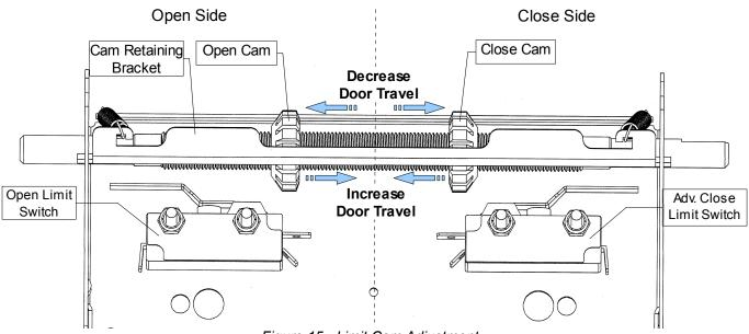
Figure 15 - Limit Cam Adjustment
