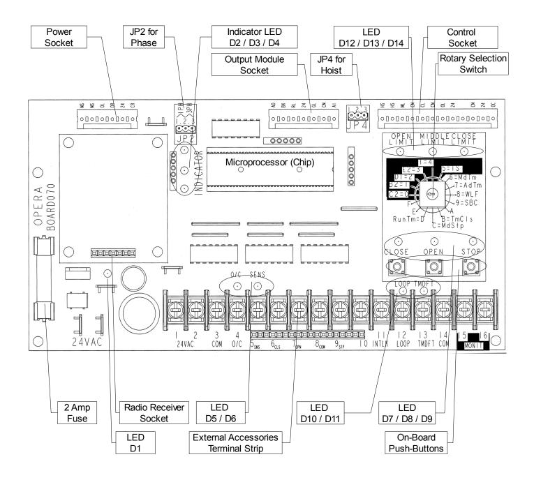
Figure 40 - Electronic Control Board – BOARD 070M
