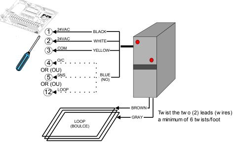
Figure 38 - Vehicle Loop Detector
