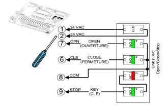
Figure 20 - STATION 080 3-PBS Open / Close / Stop with Key Lock-out and Light
