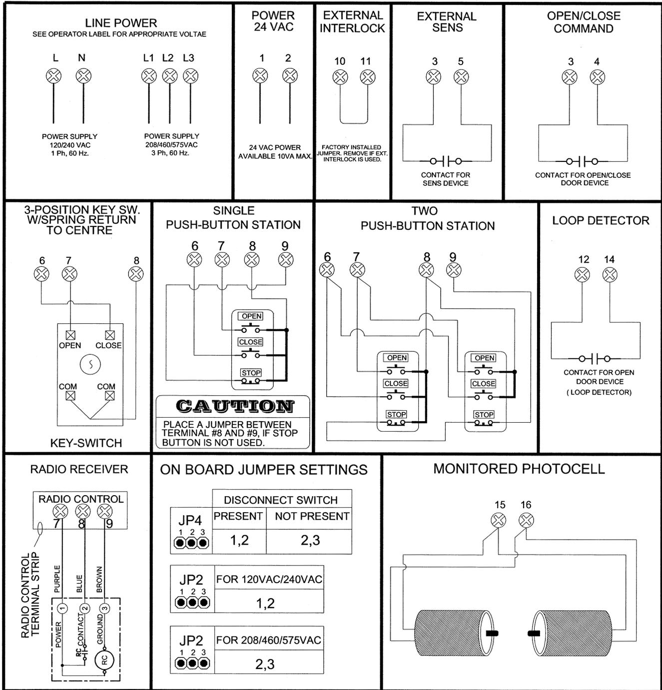
Figure 44 - External Wiring
