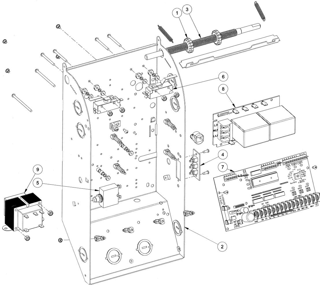
Figure 46 - Opera-GH Control Box with BOARD 070M
