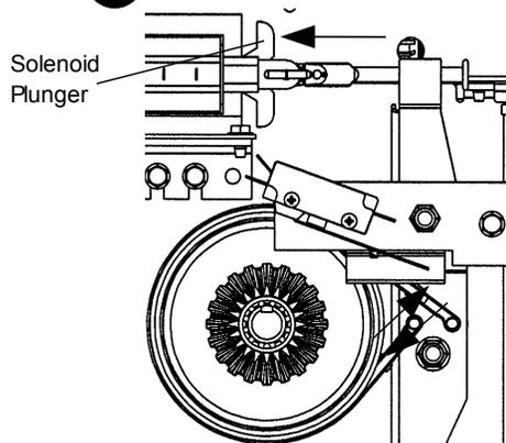
Push solenoid plunger to reduce tension when removing or installing the band brake.
