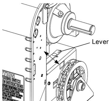
Pull the lever to adjust the gap between the plunger and solenoid body.
