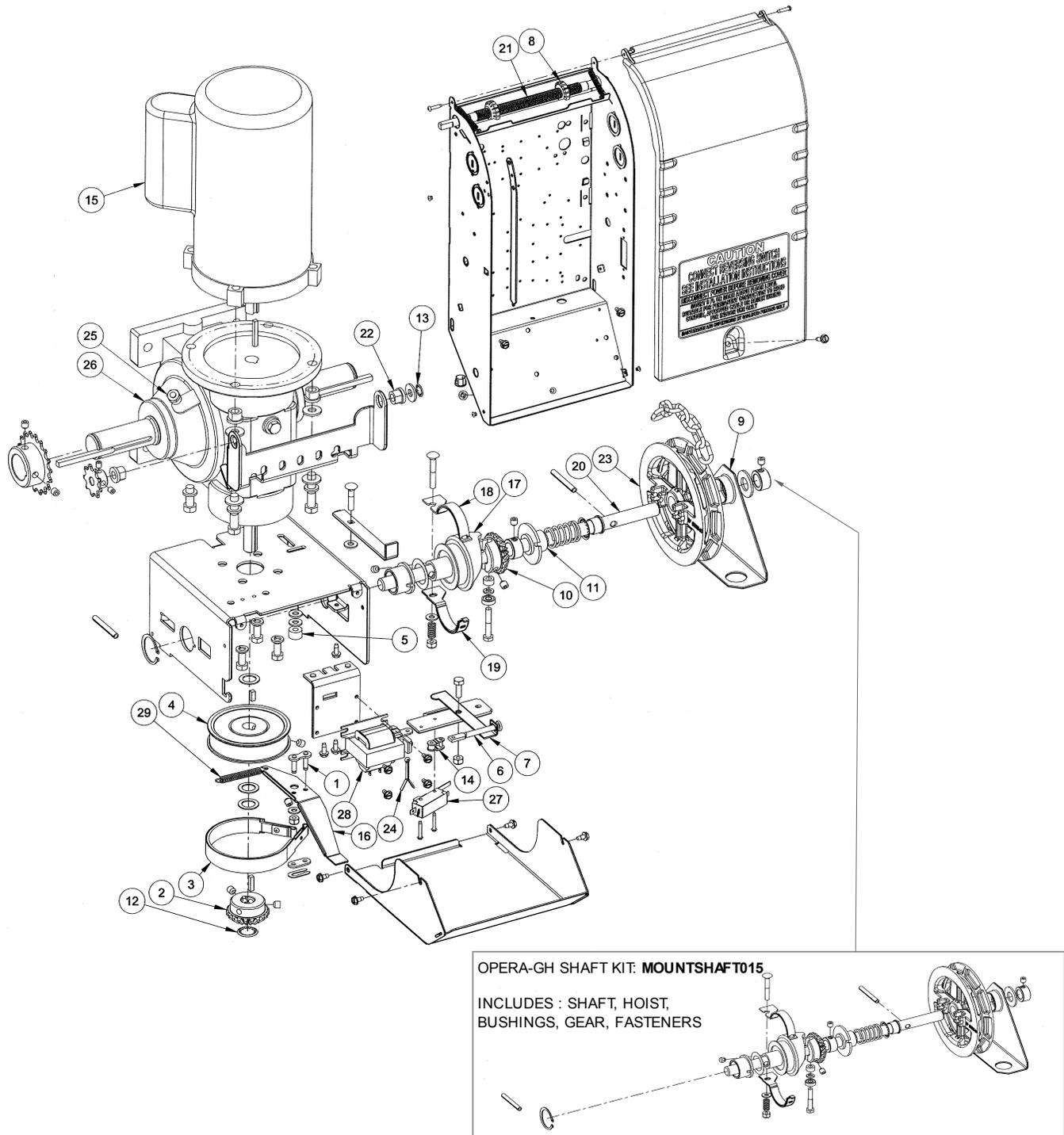
Figure 45 - Opera-GH Mechanical Exploded View
