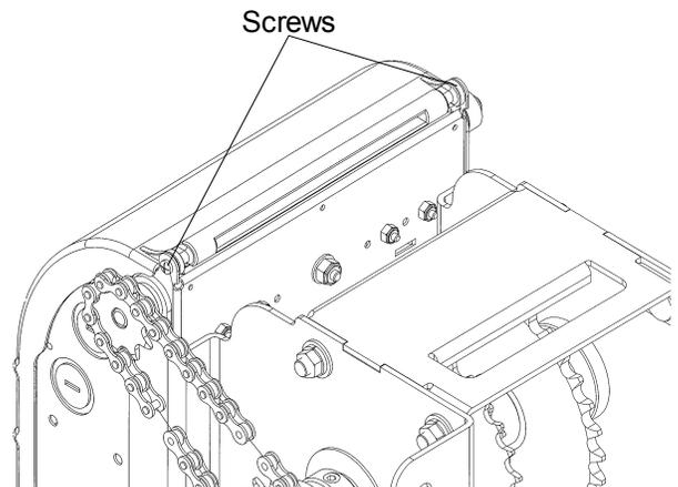
Figure 11 - Unscrewing Screws from Control Box Cover
