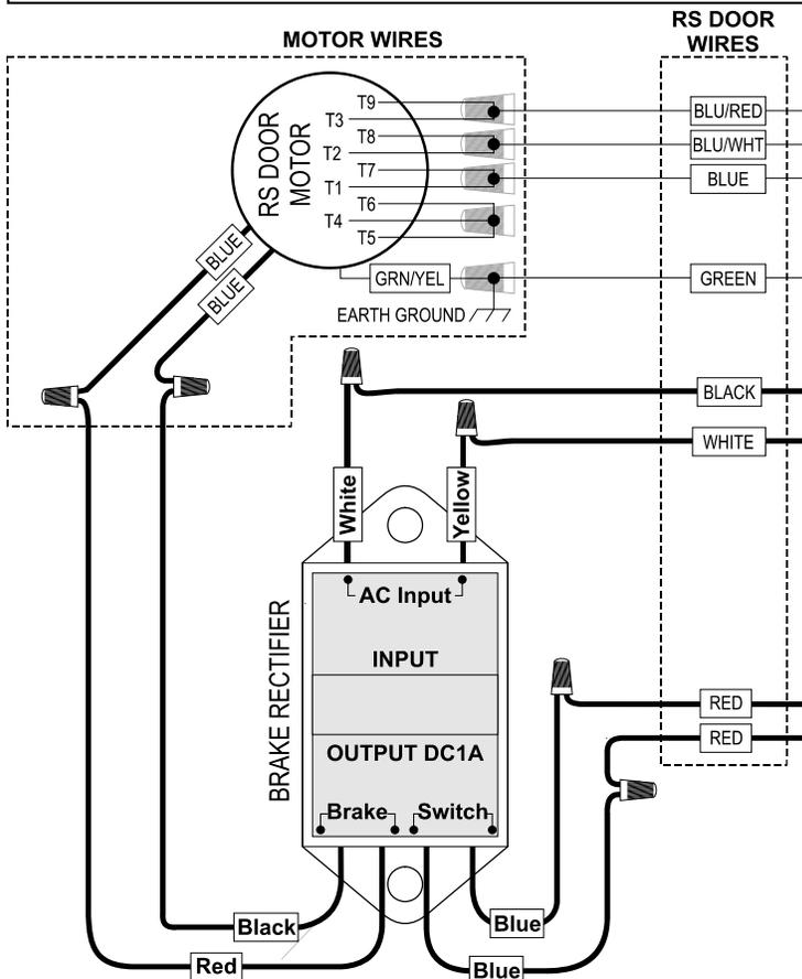
The SC-325 Controllers and RS-500 Doors can be field upgraded to accommodate either 115 VAC or 230 VAC power supply. If the desired power supply voltage is different from the factory preset/prewired voltage, the appropriate version Brake Rectifier must be ordered separately, field-installed on the RS Door, and the SC Controller switch & jumper settings changed accordingly.
