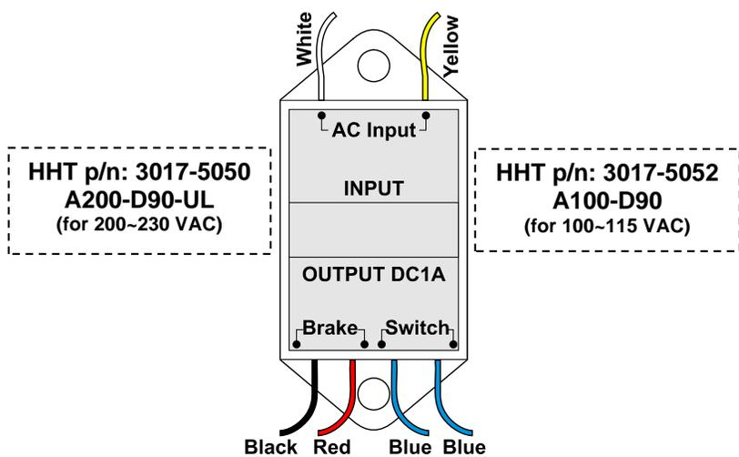
The SC-325 Controllers are factory preset to 115 VAC and the RS-500 Doors factory prewired to require a 115 VAC power supply.
