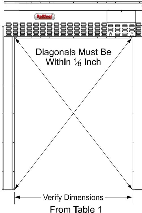
1. Use a tape measure and make sure that the overall height and overall width of the clear opening meet the requirements: Overall Height = Height + 20.688 in. (52.55 cm), Overall Width = Width + 16.4 in. (41.66 cm). Reference **Table 1, Page 3** and **Diagram 4A, Page 5**.
