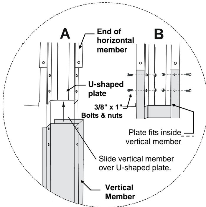
On each end of the horizontal member is a U-shaped plate that fits inside each vertical member. The U-shaped plate has four bolt holes, two on the inside and two on the outside flanges that match bolt holes in the vertical member. See **Diagram 4B**.
