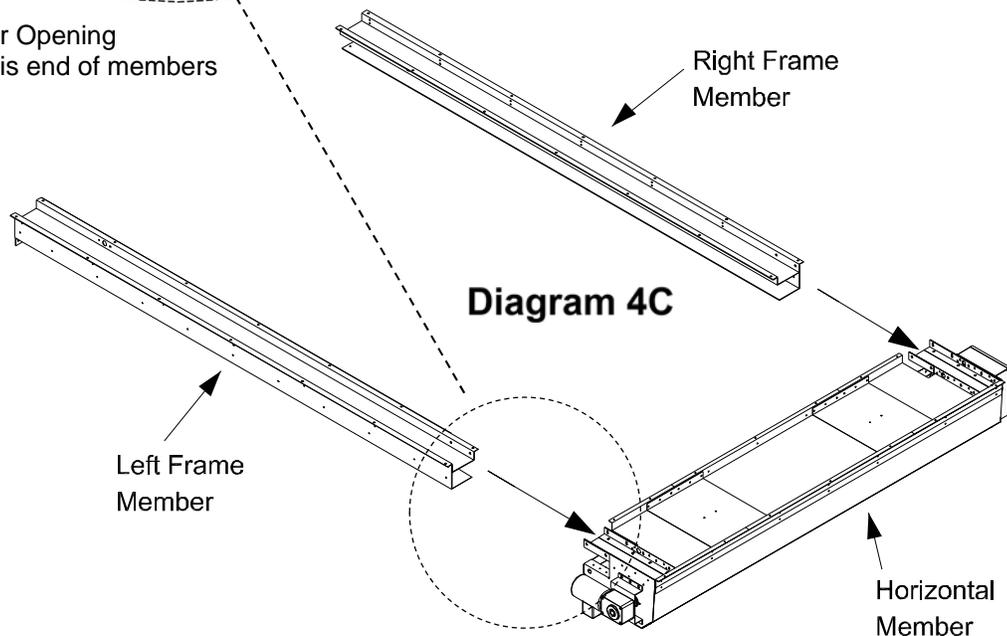
**Placement of Parts for Assembly**
