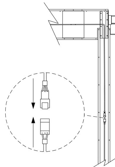
**NOTE: For each vertical member, unroll respective sensor cable attached to horizontal member until cable reaches the connector attached to the vertical member. Plug connectors together. Some slack must be left at photo eyes for replacement purposes.**
